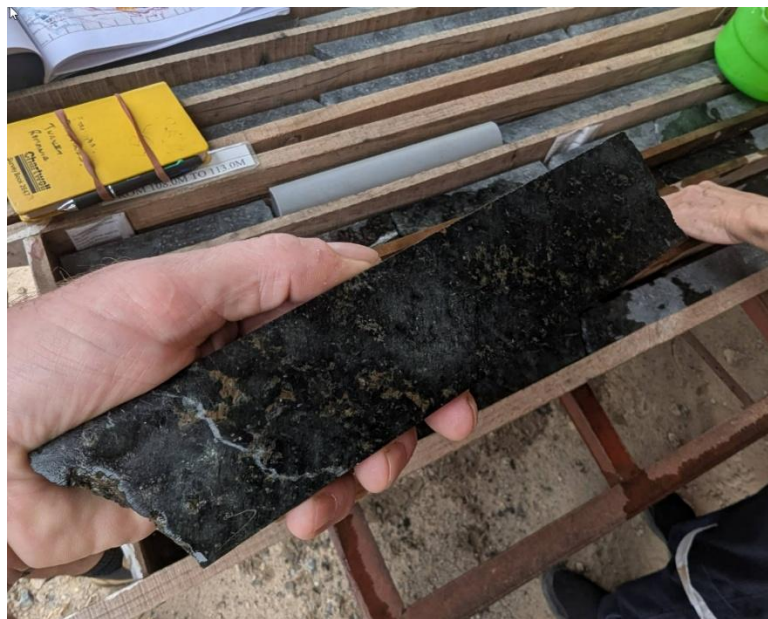
Figure 7.3_1 Disseminated Ni Sulphide Mineralisation in Ban Phuc drilling (Source Sahara 2025)
