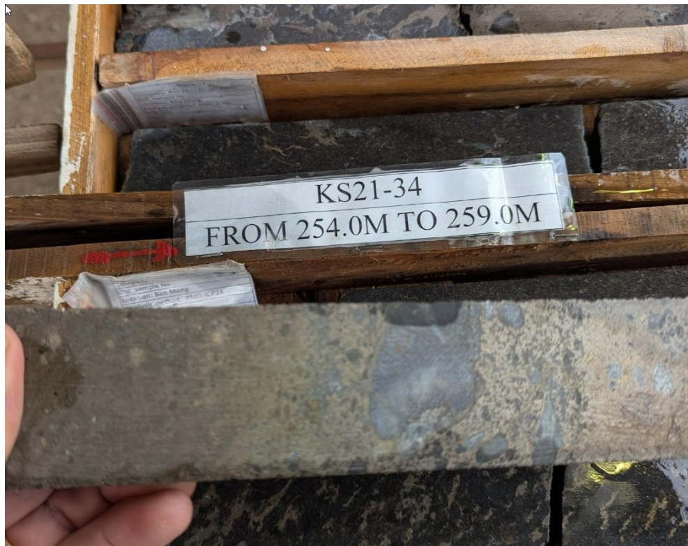
Figure 7.3_3 Massive Sulphide Mineralisation in hole KS21-34 (254m) at Ban Chang (Source Sahara 2025)
