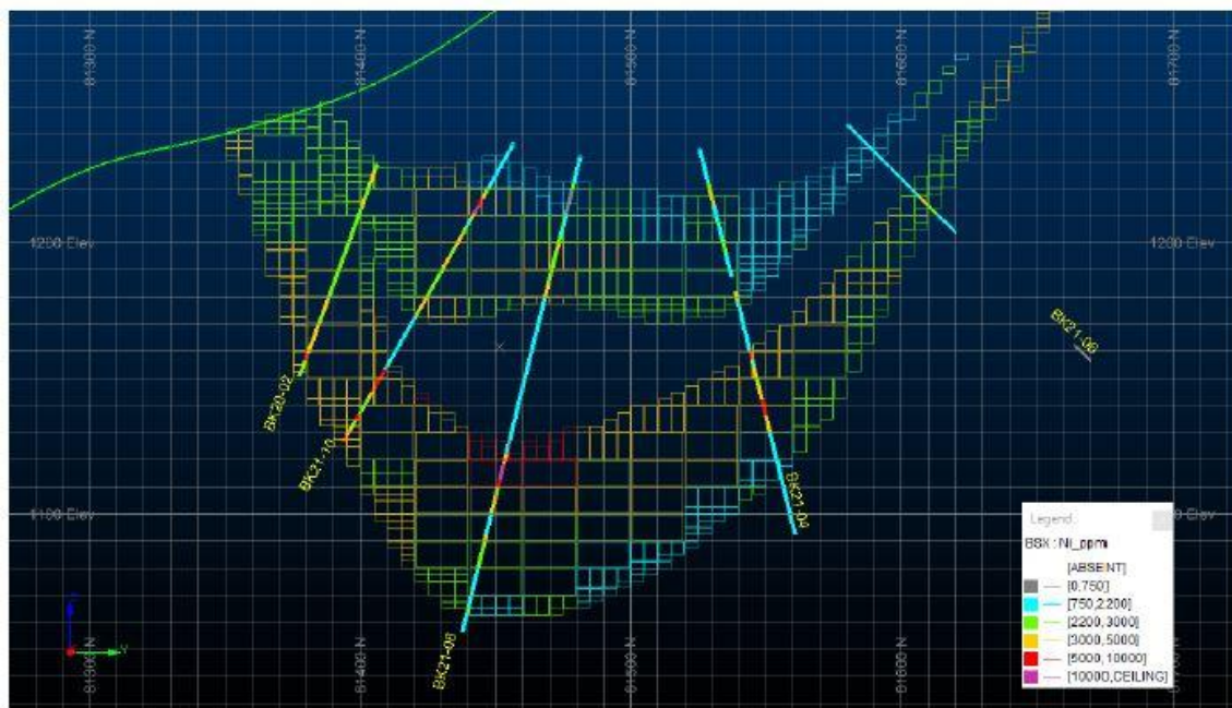
Figure 11.10.2_1 Ban Khoa cross section 49,750 mE presenting nickel grade model
