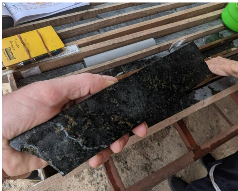
Figure 1.5_2 Disseminated Ni Sulphide Mineralisation in Ban Phuc drilling (Source Sahara 2025)
